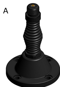
NATO 4-hole Spring 4 x M10 or 3/8" Bolts on 114mm (4.5in) PCD Base diameter 140mm (5.5in) Base height 215mm (8.5in)
