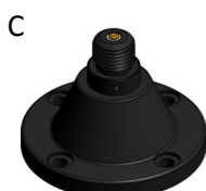
NATO 4-hole Rigid 4 x M10 or 3/8" Bolts on 114mm PCD Base diameter 140mm (5.5in) Base height 100mm (4in)
