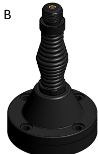
NATO 4-hole Spring GPS 4 x M10 or 3/8" Bolts on 114mm (4.5in) PCD Base diameter 140mm (5.5in) Base height 240mm (9.5in)
